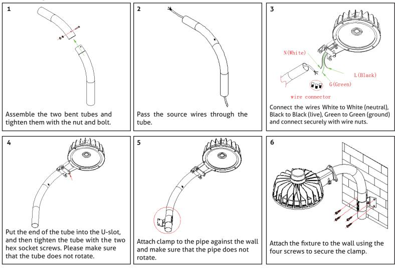
Install the light fixture on the wall with four screws through the clamp.
